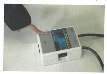
Now that you are able to operate you must then ensure that the breaker switch on the side the Quick 220 is in the ON position.
